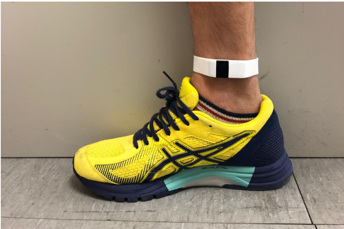
Figure 1. A wireless IMU will be positioned above the right medial malleolus by an adjustable strap.
